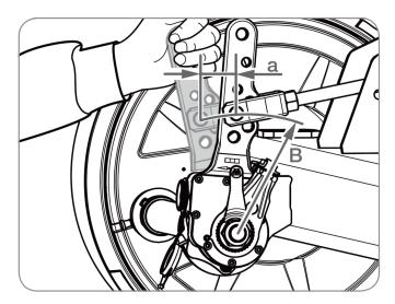
The automatic slack adjuster keeps the adjustment of the brakes in a clearly defined range to allow for normal wear and adjust the brakes accordingly
