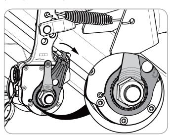
If the clevis pin movement is too little – remove the cover over the setting bolt and using a 19mm socket, depress the clutch and loosen the bolt until the movement is correct. If the clevis movement is too much – tighten the bolt.
