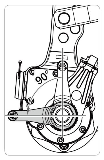
The position of the indicator will now show the remaining brake lining life. A 90° movement to horizontal indicates that the linings are worn out while a movement through 45° indicates half of the life has been used.
