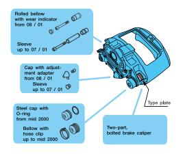
Features of the monoblock disc brake **Caliper type C**
