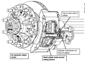
TSB Type caliper (BPW) fitted to Australian assembled axles from 05/2010.
