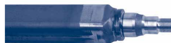
Axle beam after removing the welding flash
