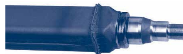
Axle beam after flash butt-welding
