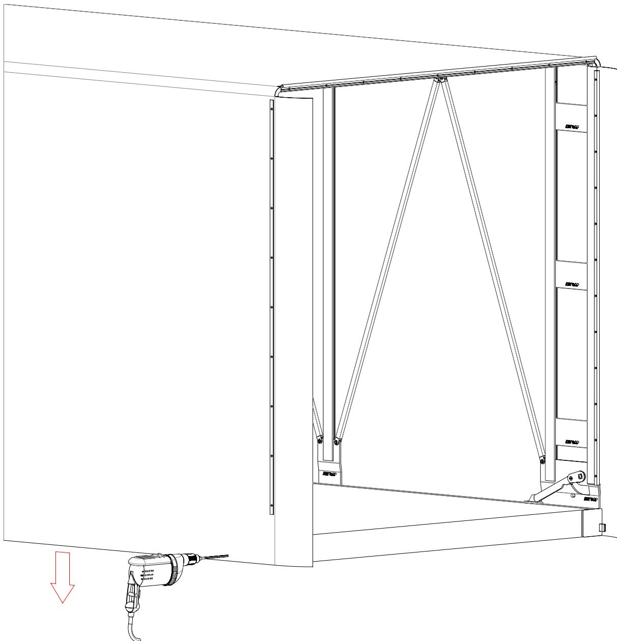
Pull down the tarp firmly. Determine the M8 threaded hole in the trolley and drill a hole through the tarp and the rubber. Install the supplied M8 bolt with large washer on each trolley.
