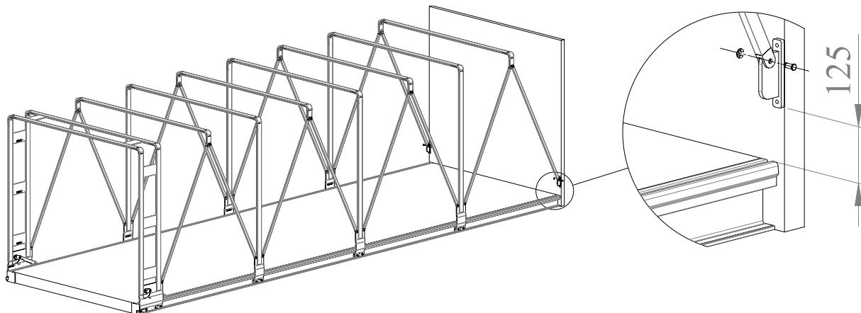
Rivet tarp on edge of headboard with alu flap 25x2
