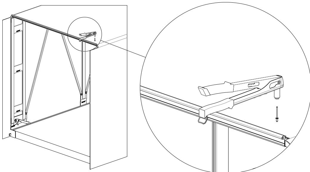
**Put L 25x25x2 profile over double layer in tarp sides and rivet**
