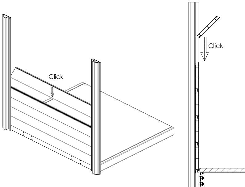
Adjust the height so the lowest plank is below the loading floor and the highest plank is 2 till 50 mm below the Netcap headboard corner post.
