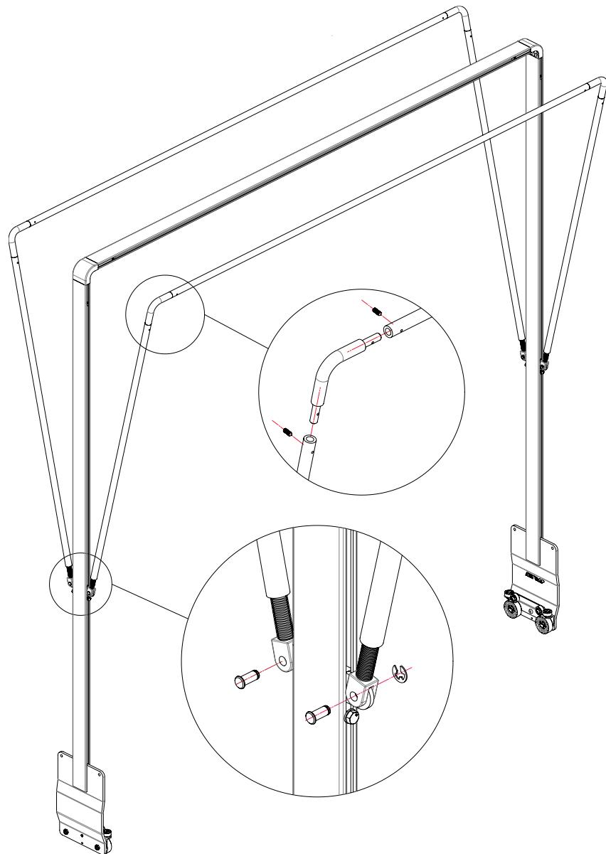
Connect each assembled lifting bow on the pre-installed brackets with a stainless bolt with groove and retainer.
