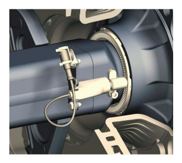
In the anti-lock brake system (ABS), the wheel movement is recorded using a proximity type arrangement with an exciter ring attached to the hub and a sensor (speed sensor) that generates the pulses.
