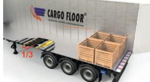
**Step 1 is repeated** moving the cargo in the desired direction. The loading/ unloading time is based on the hydraulic system, but normal cycle time is 3-10 minutes for a 13,6m trailer
