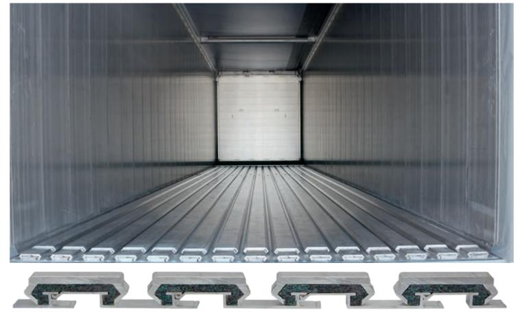
The LR-series is resistant to leaks and is NOT designated as 100% leak proof because of the undermount drive unit construction. Any leakage that may occur should only be possible at the joint between the drive system and the floor profiles. A collector bin can be installed to prevent any spilling on the floor.
