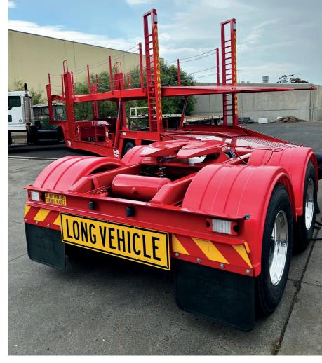
A shiny new 33-metre A-double car carrier is going to hit the Tasmanian roads soon. Custom-built to meet Performance-Based Standards requirements, the new combination was manufactured using BPW drum brake axles and suspension – a combination trusted by North Geelong-based Pacific Trailers for over two decades.
