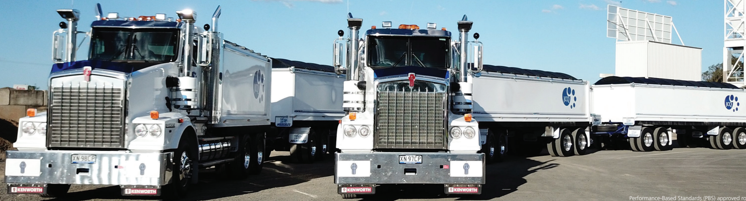
Performance-Based Standards (PBS) approved road train combinations fitted with BPW disc brake axles and heavy-duty suspension to manage difficult terrain and rough roads.
