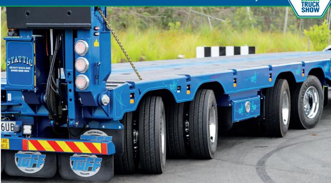
built-up areas. Our new quad axle low loaders give us that edge we need to navigate such places. The steering gives us excellent manoeuvrability, which is so important when you're moving heavy equipment. There is also less wear and tear on the tyres. When you're moving 40-50 tonne equipment, narrow spaces like what we work in can be very rough on the tyres but the steering movement with our BPW axles makes it easy for the trailer and also the driver to navigate."
