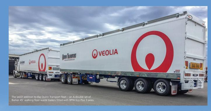
One of the latest additions to the Quinn Transport fleet is an A-double set of Barker 45' walking floor waste trailers fitted with BPW Eco Plus 3 axles. Along with the new set of Barker trailers, Scott purchased a new set of Byrne Livestock B-double crates, also with the BPW Eco Plus 3 axles. componentry shows that the secondgeneration family business is committed to delivering a consistently reliable and quality service across its diverse transport portfolio.
